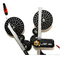
**Manipulator B:** Student has supplies to build manipulators that involve servos. They use the programmable servo to power and test the servos in their manipulator.
